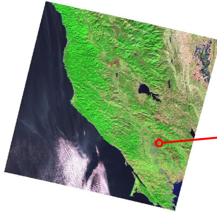
Changed brightness, gamma and contrast and applied new bandwidth combination to show burnscar (7,5,4 shortwave infrared)
