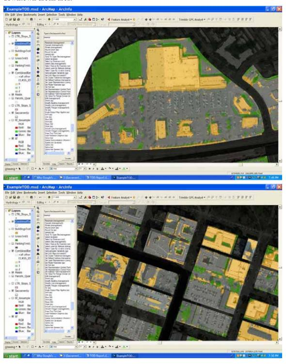
16) The next step was to use Hierarchical Learning to begin removing clutter from the image and tag areas that were classified incorrectly. Each classification was separated out with each class going through the clutter removal process. Approach 2 was utilized because it was recommend in the software manual for removing clutter. Again, a square input analyzer was used given the configuration of the features being classified. Below is the building classification after the clutter procedure.
