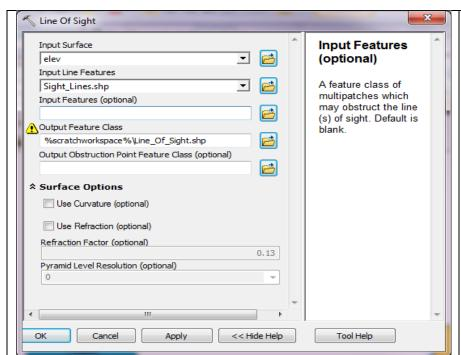
The Line of Sight uses the surface raster and the sight lines created above to create the surface hugging red lines shown in the ArcScene image above.
