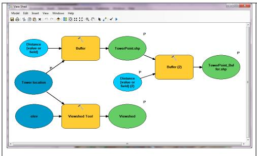
The viewshed and buffer model uses a "mouse click" as input for the proposed tower location and builds a viewshed with shapefile, rather than raster, as an output type.
