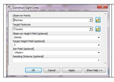
As you can see from the Line of Sight model above, the model first creates 3D sight lines between the observer points and the target features. These are the straight black lines shown in the ArcScene image above.
