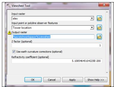
The viewshed parameters require an input elevation raster, an observation point and an output location for the viewshed raster that would be created.
