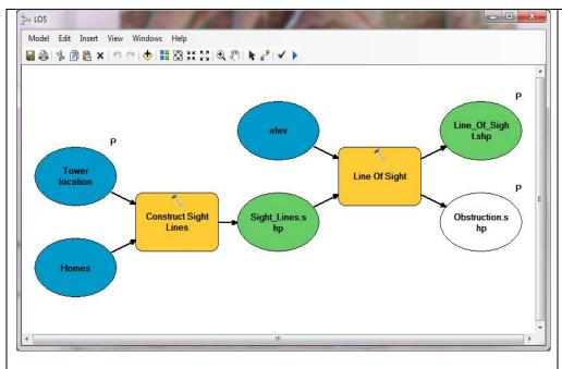
My Line of Sight model was initially setup to use the tower point shape file that was created in my viewshed model but I kept getting file sharing errors until I revised it to use an input variable just like the other model used. The user simply clicks the mouse on top of the point created with the viewshed application.
