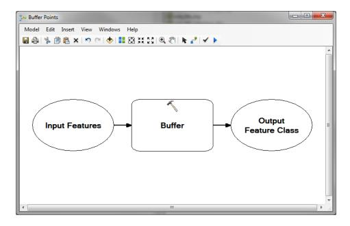
Right-click Input Features and select properties. Click the Data Type tab and choose Feature Set from the Select data type drop-down list. On the Import schema and symbology from box, browse to the "Points" feature class within the Schema geodatabase to find and set the data-path to the data for the Input Features variable.
