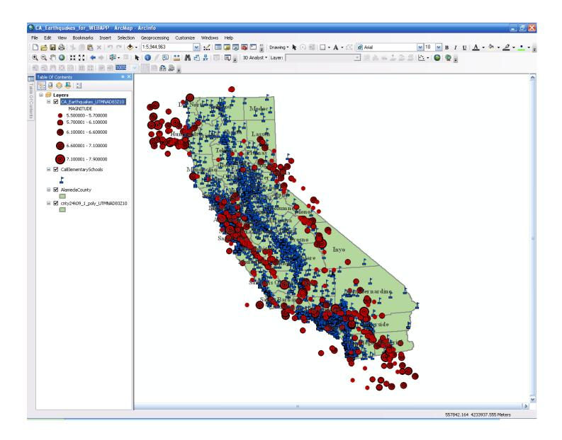
After the symbology, layer visibility scale range, and the layer labeling scale range have been set, go to File in the Arcmap menu taskbar and click on Map Document Properties. On the Pathnames tab, check the Store Relative Pathnames to Data Sources option, and save the map as CA\_Earthquakes\_for\_WEBAPP.
