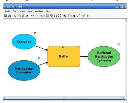
In the main ModelBuilder menu, click Model and click Model Properties. Set the name to BufferPoints, set the label to Buffer Points, and make sure that the Store relative path names option is checked. Click OK.
