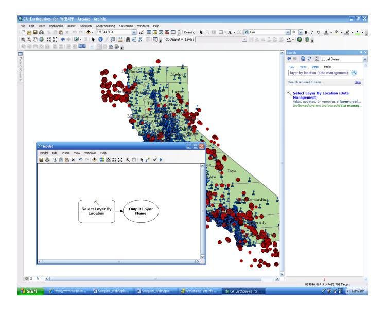
Right-click the Select Layer by Location variable then go to the Make Variable From Parameter option and select Input Features. Right-click the Select Layer by Location variable again but this time go to the Make Variable From Parameter option and select Selecting Features.
