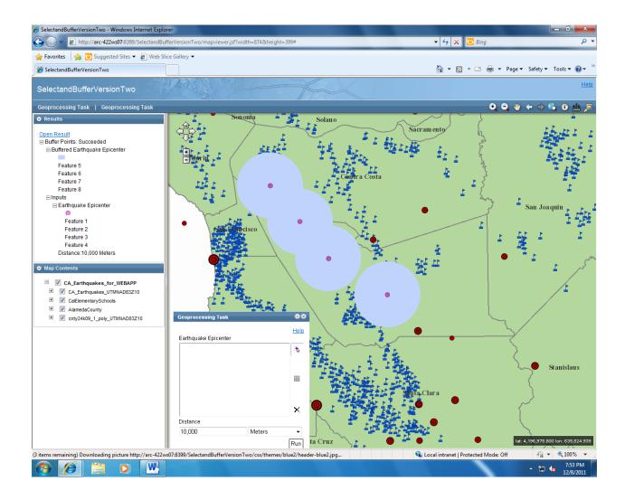
Next, the user clicks on the second Geoprocessing Task, this is the AlamedaCountySchools geoprocessing task that will select all the Elementary schools in Alameda county when the geoprocessing tool is run. When the user clicks the second Geoprocessing Task, the Geoprocessing Task dialog box opens.
