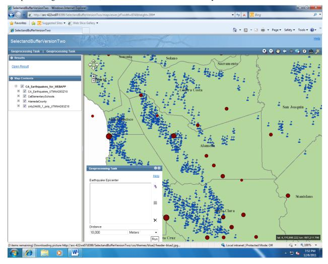
The Buffer Points geoprocessing task dialog box opens to allow the user to interactively select the points to be buffered.
