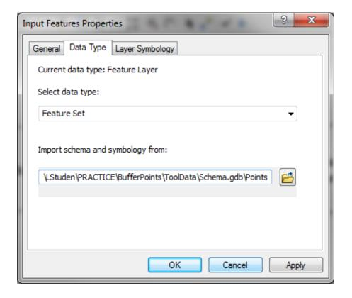
Click OK. Right-click the Buffer tool and point to Make Variable From Parameter to create a new model variable. Click the Distance [value or field] option from the Make Variable From Parameter menu, this creates a new variable named Distance [value or field]. Right-click the newly created variable and rename it "Distance".
